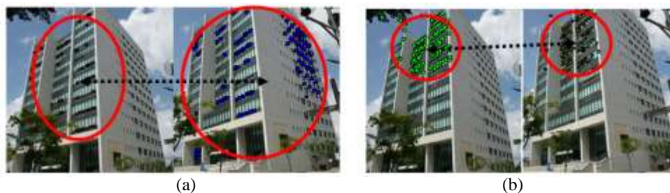
Figure 5. (a) Matching between clusters generated from conventional clustering (b) Matching of clusters from two-step clustering (Red circle represents a rough area of keypoint distribution)
